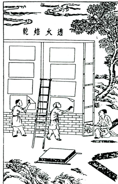
Chinese paper-making. From T'ien-kung k'aiwu , a dissertation on crafts by Sung Ying-hsing, 1634. Top left: Steaming bast. Top right: Paper formation. Bottom left: Pressing. Bottom right: Drying against a heated wall.
