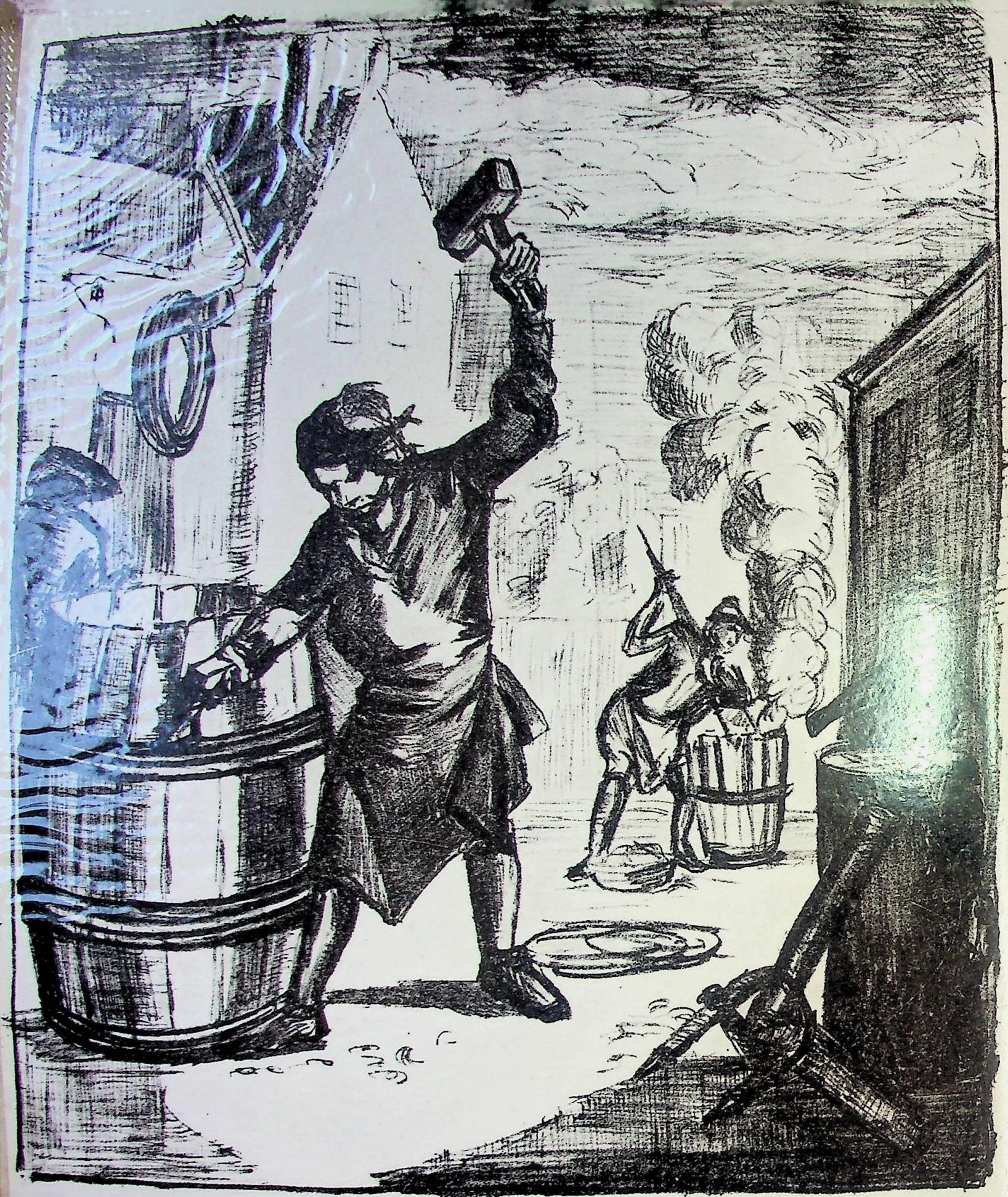
Plate I - 16<sup>th</sup> Century cooper at work - the figure in the foreground is using a maul and driver. To the right of the picture is an axe in a notched block - a cleaver against the block and a compass resting on the ground. In the background a cask is being fired, in preparation for bending and driving -
