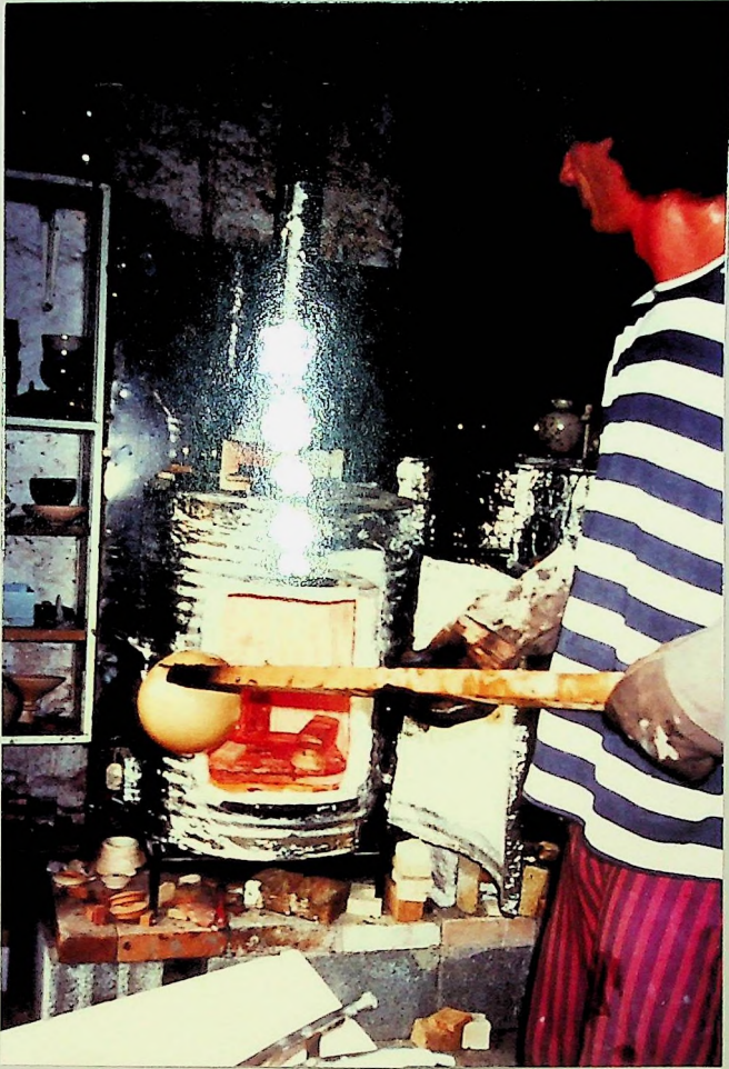
Fig.1 Removing pots from the Kiln.
