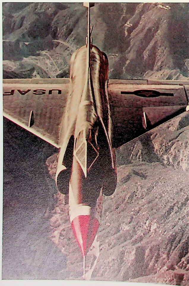
Fig.16(below): Convair F-102A Delta Dagger. Note 'waisting' of the fuselage- a feature of area-rule.
