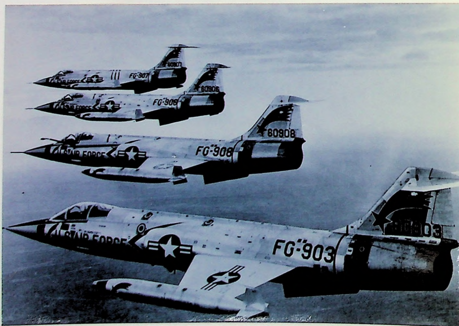
Fig.17A: Four Lockheed F-104C Starfighters. Note extremely long and pointed fuselage, stubby wings and wing-mounted fuel-tanks.
