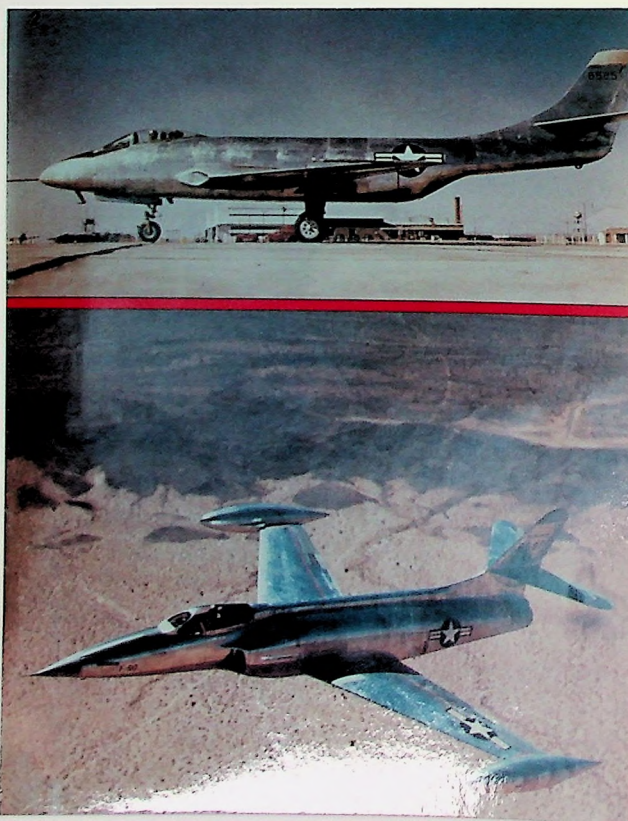
Fig.14(below): McDonnell XP-88 and (bottom), Lockheed XP-90. Note dramatic dart-like form of the Lockheed design. The XP-88 was finally ordered as the F-101 Voodoo.
