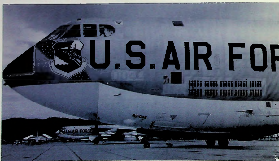
Figs.26&27: Note enlargement in SAC badge and U.S. AIR FORCE legend apparent from earlier 1954 B-52A(top) and 1958 B-52D (above). B-52D also has white underbelly.
