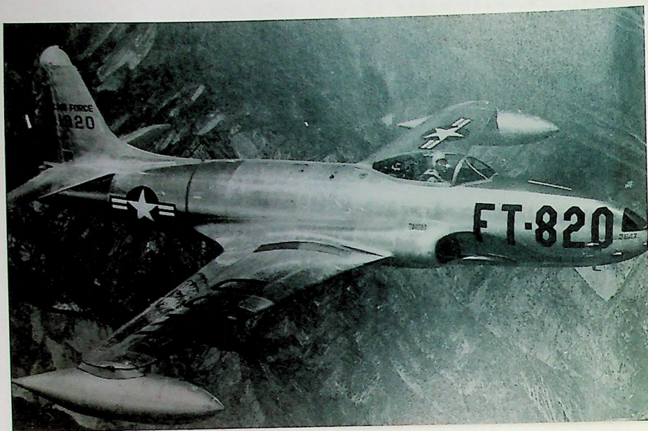
Fig.3: Lockheed P-80C Shooting Star. It's clean form and straight wings are clearly shown.
