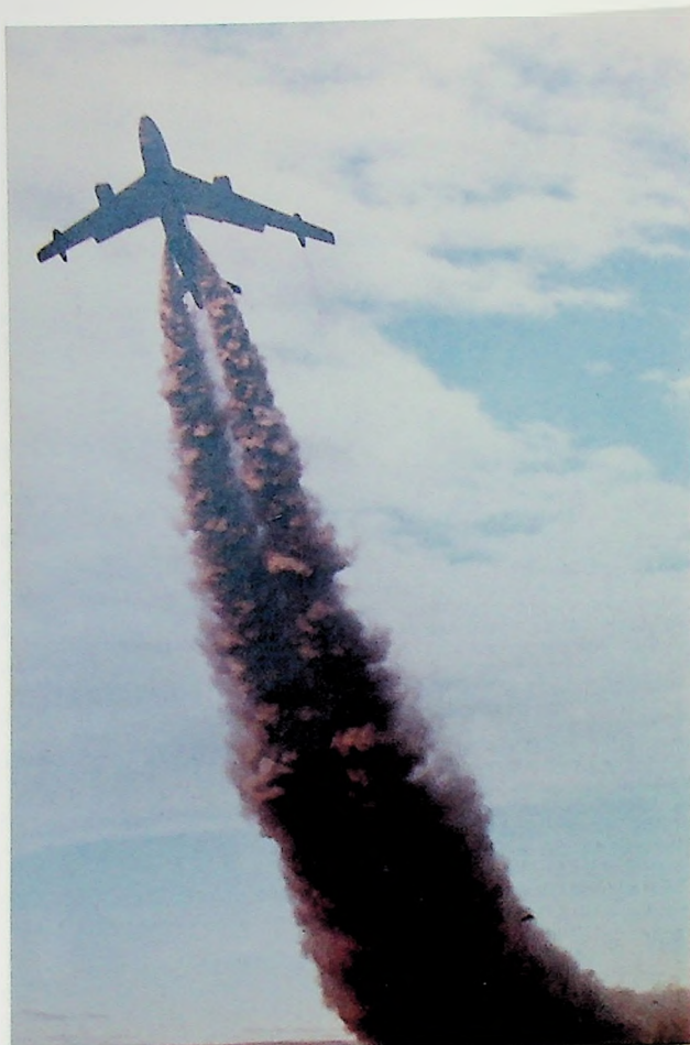
Fig.11: B-47C Stratojet taking off with full rocket-assistance (JATO).
