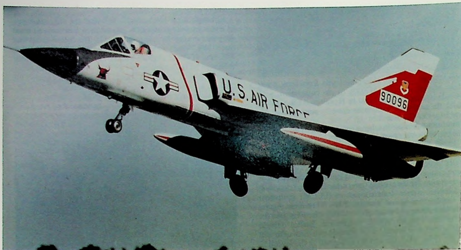
Fig. 17: Convair F-106 Delta Dart. Although superficially similar to the F-102A, the F-106 was a completely new aircraft with Mach 2,4 performance.
