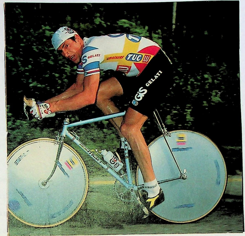
Fig 26 FRANCESCO MOSER RIDING HIS LOW PROFILE BICYCLE WHICH HE USED FOR HIS HOUR RECORD.
