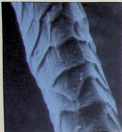
Wool fibre after treatment by chlorination resin process. Scale structure is still apparent but masked by a layer of polymer.
