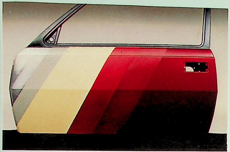
14 layers of primers and paint for lasting protection
