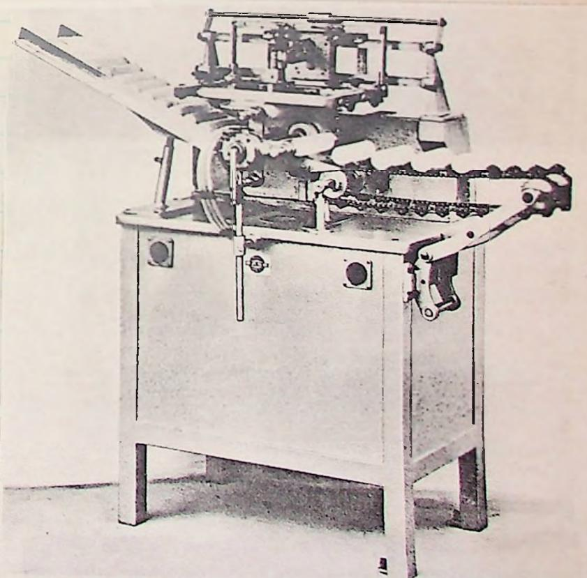
FIG. 83. Fully automatic turret printer designed for high-speed screening on cylinders. It features a multicolor registration device and an automatic inflating device for soft wall plastic containers. (Courtesy American Screen Process Equipment Co.)
