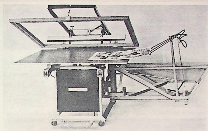
FIG. 93. The Filbar Press, with automatic take-off device. Its versatility permits it to print on both rigid and flexible material at speeds adjusted to the nature of the material. It is comparatively inexpensive but sturdy in construction. (Courtesy Graphic Equipment of Boston, Inc.)
