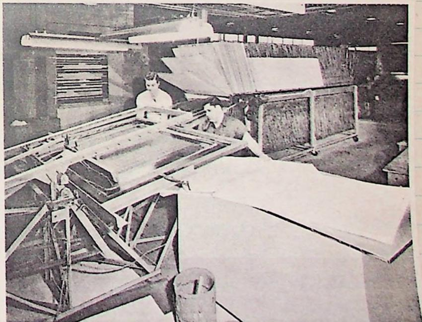
FIG. 119. View of printing department, showing automatic printing and drying equipment in use.
