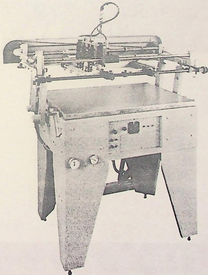
FIG. 94. The Precision Industrial Screen Printer, versatile but especially well suited for screening printed circuits and other industrial fabrications. (Courtesy Precision Screen Machines Co.)
