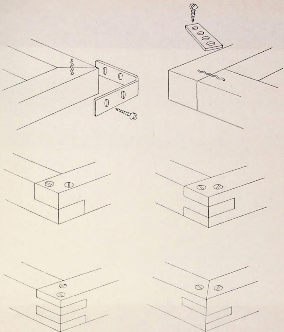
1.2 Various joints used for screen frames. From top left: miter, butt, lap, simple tongue-and-groove, double tongue-and-groove, miter tongue-and-groove.
