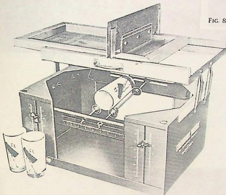
FIG. 82. The "Streamliner," a screening set-up for printing on large cylindrical objects. (Courtesy Atlas Silk Screen Supply Co.)
