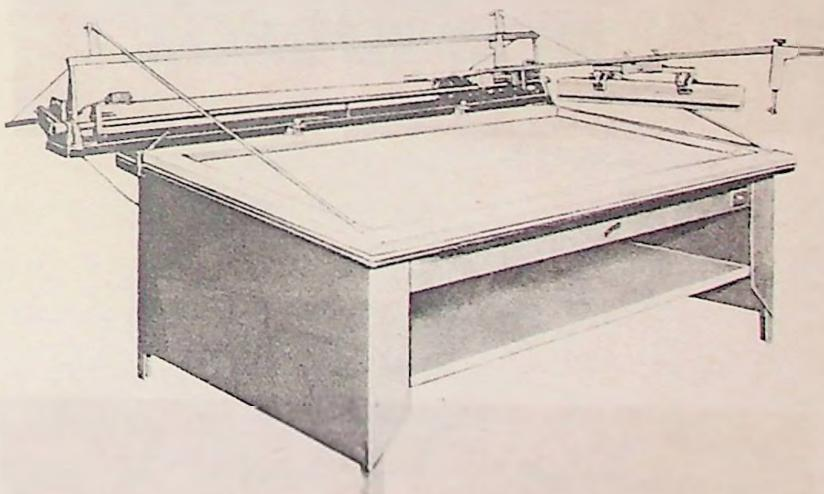
FIG. 95. The "One-man squeegee," an efficient manual printing unit with a patented counterbalanced squeegee device. (Courtesy Cincinnati Screen Process Supplies, Inc.)
