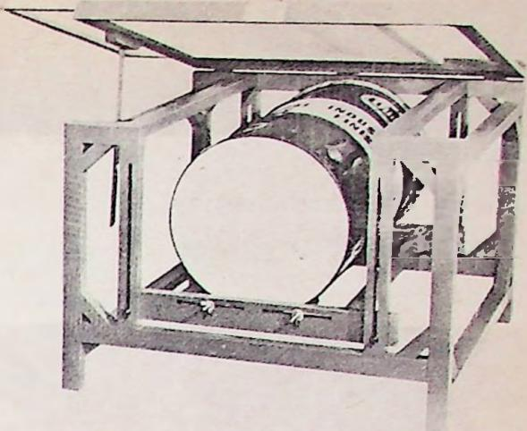
FIG. 81. The "Sparky" jig, a simple device for screening on round objects.
