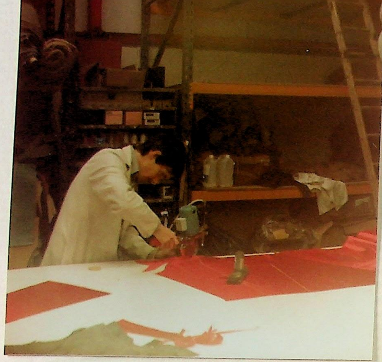
lining is cut out
