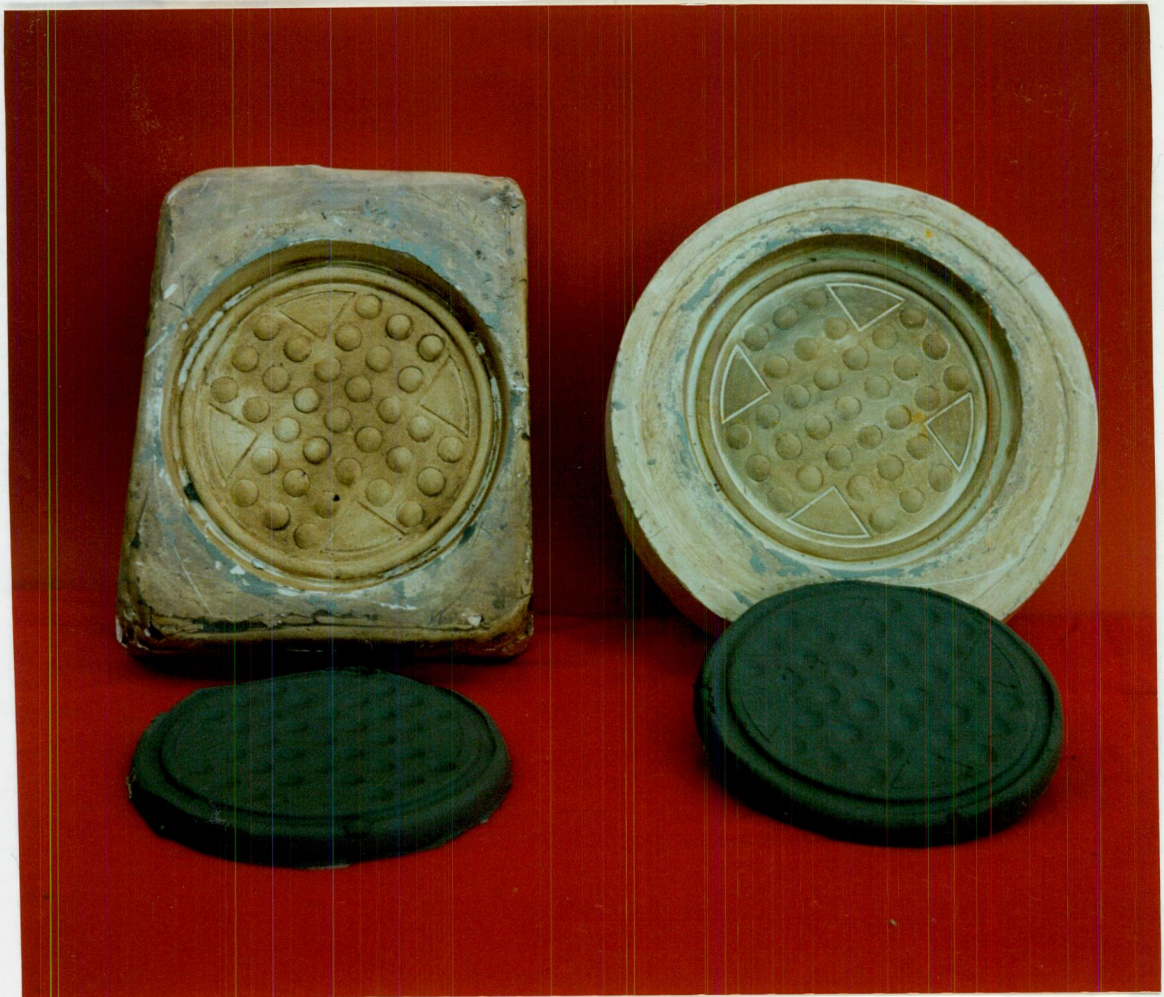
7.TWO SOLITAIRE WERE MADE TO SPEED UP PRODUCTION PURPOSES, ABOVE ARE THE TWO MOULDS WITH TWO FREASHLY CAST GAMES BOARDS
