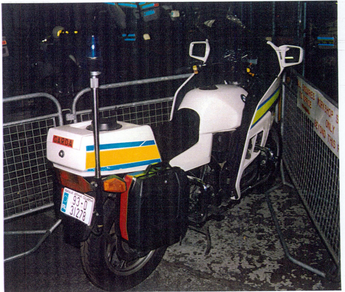
Plate 6; Rotating beacon bolted on to the rear mudguard and pannier of a BMW authority motorbike. Note also the two crash bars which are attached perpendicular to the motorbikes length. The rear panniers can be seen, the top one containing the radio.
