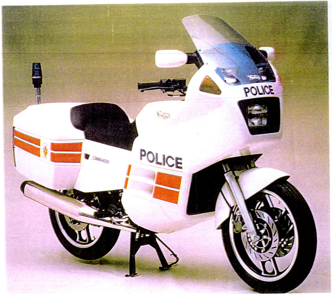
Plate 20; The identification lights are integrated into the front fairing, the sirens and crash bars are integrated into the body underneath the Commanders shell. The finish is very clean with very little styling.
