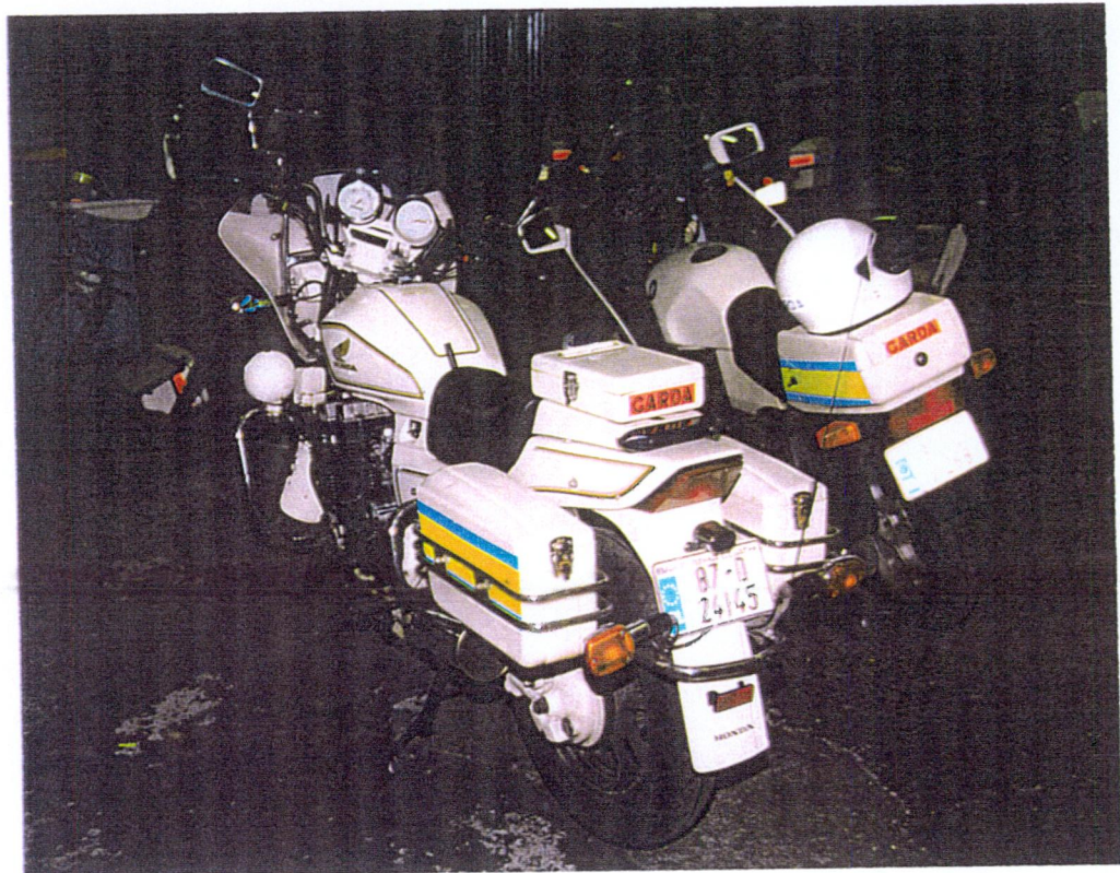
Plate 14: Honda CBX police special showing panniers and chrome detailing. Note blue light and clip on top of the top pannier for holding tickets.
