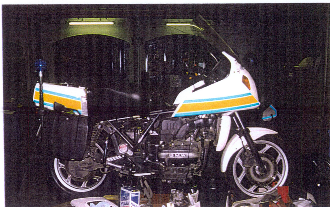
Plate 9: BMW authority motorbike during maintenance, the side fairings, side panniers, and part of the front crash bars have been removed and the seat hinged up.
