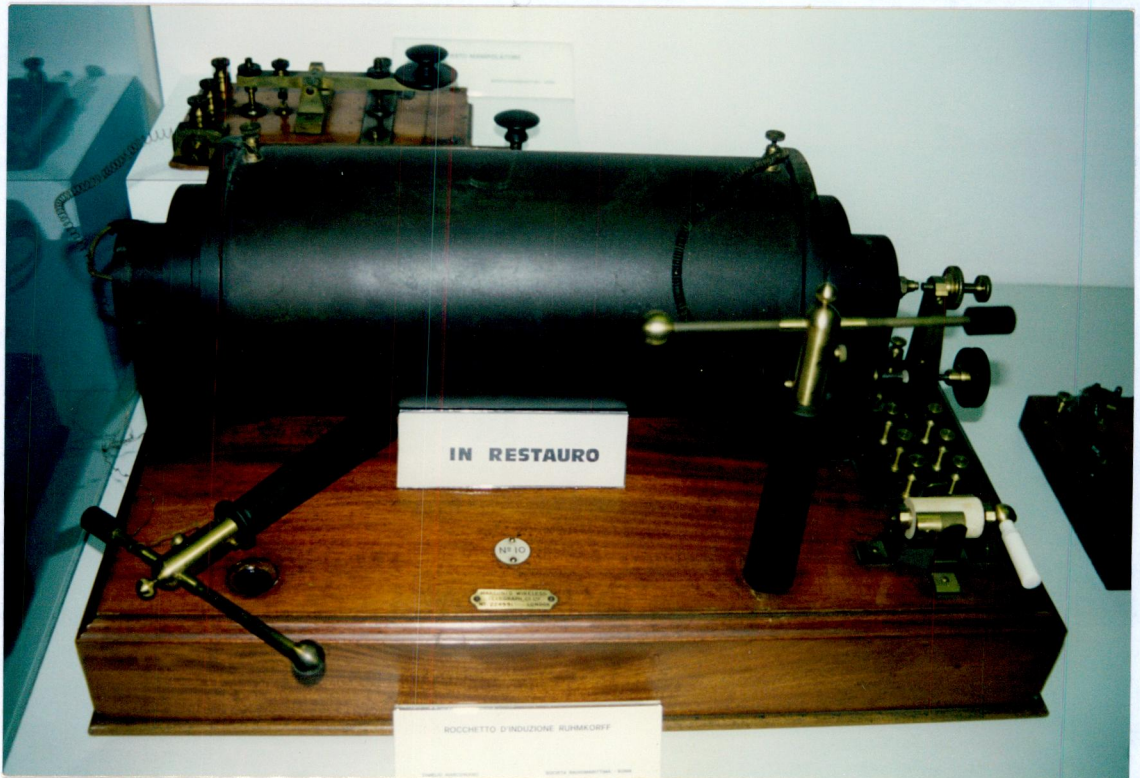
Fig. 6a. The Ruhmkoff Coil. ( Transmitter ).
