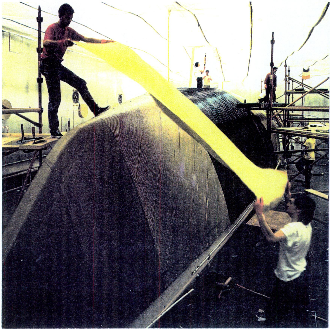
Fig. 17. Building "NCB Ireland's" composite hull.
