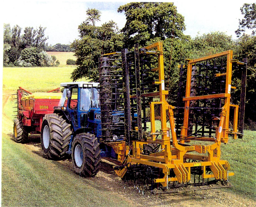
fig30 A Ford 8730 in transit with a row harrow attached to the front and a trailed seed drill behind and below, the same tractor at work in the field.
