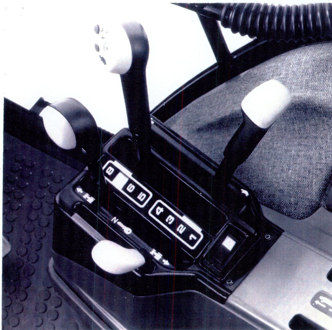
fig.5 Ford ElectroShift transmission system, 1991
