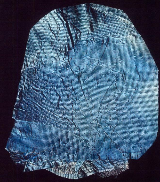
MAIN PICTURE THIS PAGE & OPPOSITE: Arai's recent experiments include slit-film metallic fabrics which are hot-pressed into semi-rigid irregular plates, sometimes 50 cm across - the one pictured is 8 cm. Each side is a different colour. The larger lightweight plates have been used as armour-like
